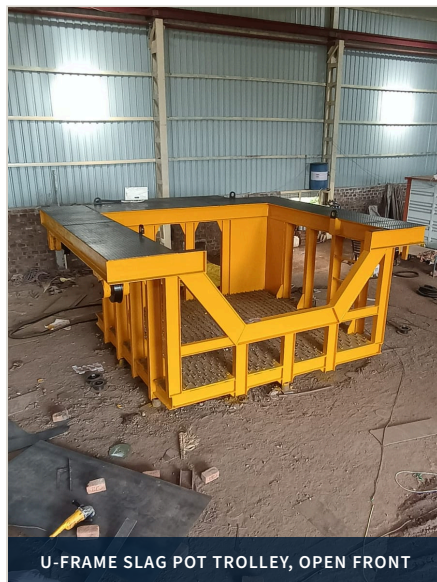
SLAG POT TROLLEY, 30 T SWL, GEARED DRIVES
