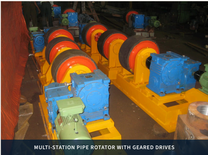
PIPE ROTATOR, ADJUSTABLE ROLLER CENTRES
