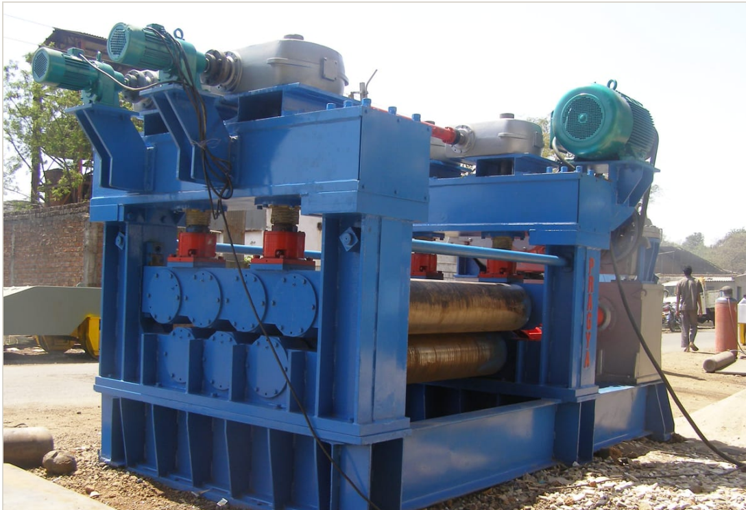
PLATE LEVELER Thickness 0.13-152 mm
