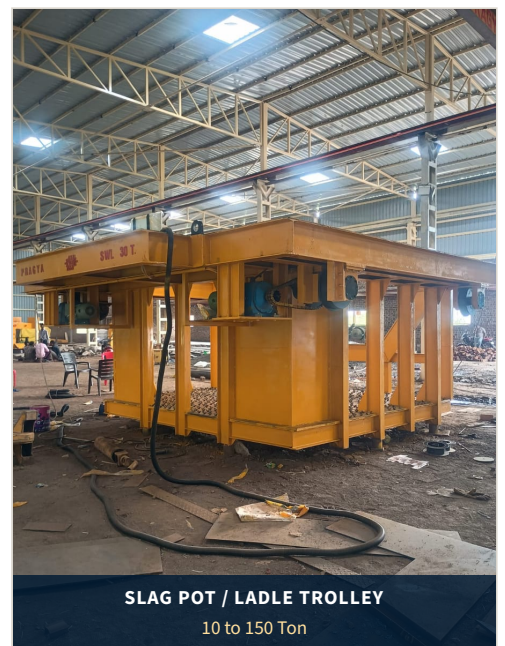
TROLLEY WITH TILTER 0-90° Hydraulic Tilting
