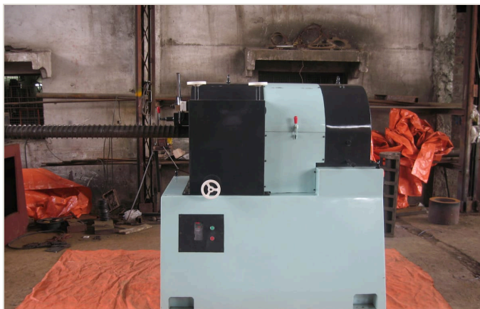
DRIVE AND CONTROL SIDE Tube OD 8.0 to 100 mm, fin pitch 2.0 to 10.0 mm FPI
