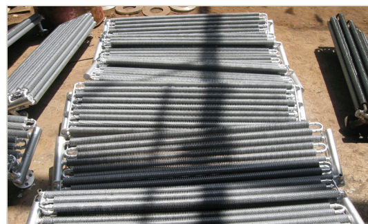
FINNED TUBE ELEMENTS WITH RETURN BENDS Tube OD 15 to 220 mm
